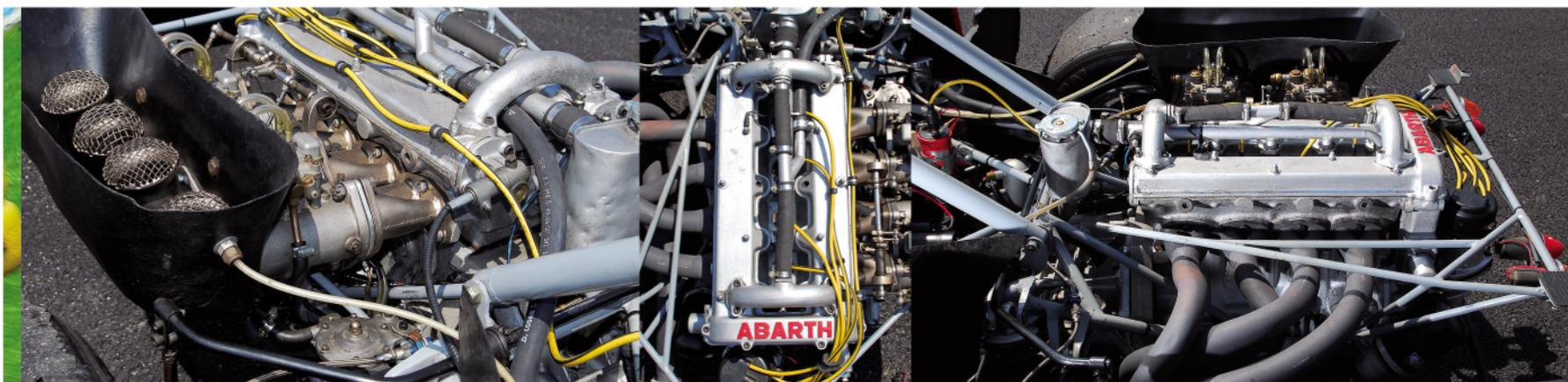
**ABOVE:** The superb 2-litre twin cam engine produces 250bhp at 8000rpm. With the Abarth weighing in at just 530kg the power to weight ratio is an excellent 472bhp per tonne
